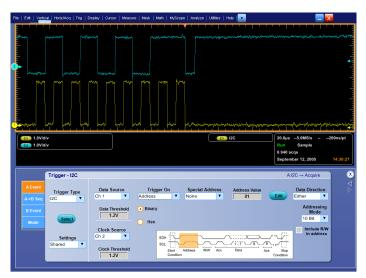
Easily trigger on a specific I<sup>2</sup>C address.
