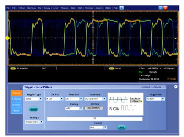
Serial pattern triggering to debug pattern-dependent issues.
